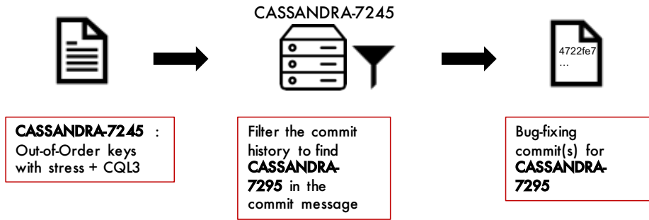
Fig. 4: An overview to extract fix commits given the JIRA issue ID: CASSANDRA-7245.
